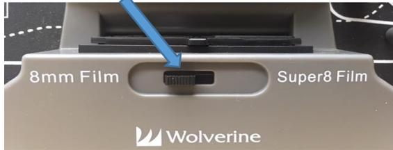
It is important that you select the correct film type. If you are unsure, look at the notched holes on your film. The holes for 8mm are off-set. The holes for Super8 are centered.
