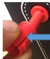
**Note:** If your reel has a large hole, you will need to attach the red reel adapter to the red spindle
