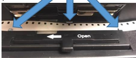
8 Continue routing your film along the white line and insert the end of your film into the notch on the empty take-up reel, manually turn the reel about one rotation
